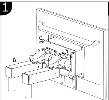
Attach VESA plate to monitor using Phillips pan head screws (C).
