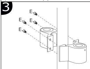
With the proper bushing or insert in place, attach the mount to the pole using a 3/16" Allen wrench and four 1/4-20x1/2" screws (E). To ensure a proper fit, first install all 4 screws without over tightening. Then gradually tighten each screw a little at a time, moving from one screw to the next to keep the pressure relatively even.
