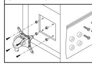
.25" Spacer Hardware Kit (4) .25" Spacers (4) M4 x 18mm Phillips Pan Head Screws Order # P404923-B
