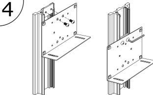
To track mount, thread the bolts through the backplate and into the slider plate a few threads. Once in preferred position, level the plate and tighten the bolts to secure the plate to the track. Attach the front plate as in Step 1.
