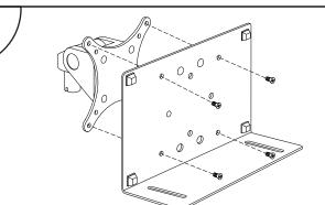
The back plate can be mounted directly to a vertical surface (using fasteners provided by customer) or, as pictured, the back plate can be attached directly to a Vesa plate on the tilter head. Attach face plate as in Step 1.
