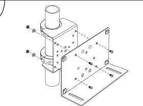
To pole mount, attach the backplate to the universal mounting bracket, using provided fasteners. Then attach the face plate as in Step1.
