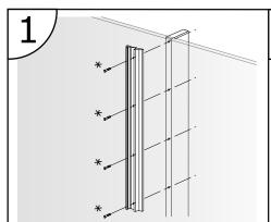
Align track mounting holes with wall stud. Be sure to fasten the track directly to a wall stud.
