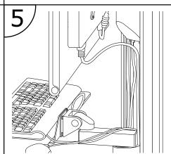
Run wires and cords from devices behind the track mounts and out either end of the track.
