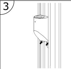
Secure by tightening the set screws provided with each component.
