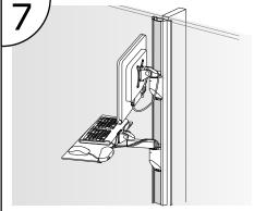
Insert the covers into the track mount slots. Place one edge into one side, bend slightly. Then starting at the top, pop the other edge in, working the way down.
