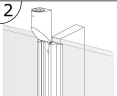
Slide track mounts (or other Ergomart brackets and components) into the track slots from either end of the wall track.
