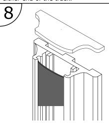
Press end cap onto each end of the wall track.
