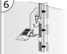
Cut the plastic wire management strip into lengths about one half inch shorter than the spaces between the mounts and/or the ends of the wall track.
