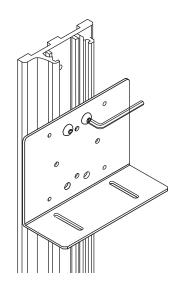
Position the CPU back plate on the track, level it and then tighten the bolts to secure it to the track. Use the fasteners provided with the CPU holder to attach and adjust the front plate.
