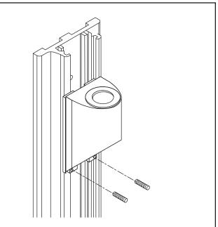
Secure mount by tightening the set screws provided.
