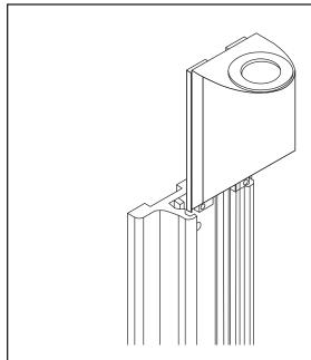
Slide track mount into the track slots as shown.
