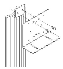
Attach the CPU holder back plate to the vertical slider plate using the provided bolts. Leave the bolts loose enough to slide the plate along the track.
