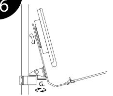
Increase resistance to tilt by adjusting set screw at the point of articulation using wrench (G.)
