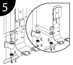
Slide tilter pin into the wall mount and secure with dog washer (E&F.)
