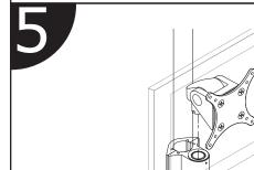
Place tilter head with monitor in mount and secure with dog washer and screw.
