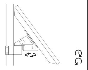
Adjust tilt resistance using 3/16" Allen Wrench.
