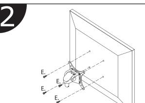
Attach monitor to VESA plate using Phillips pan head screws.
