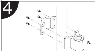
With the proper bushing or insert in place, attach the mount (B) to the pole using the included four 1/4-20x1/2" screws. To ensure a proper fit first install all 4 screws without overtightening. Then gradually tighten each screw a little at a time, moving from one screw to the next to keep the pressure relatively even.
