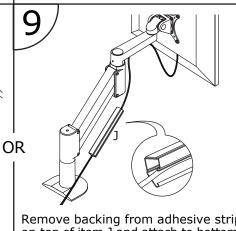
Remove backing from adhesive strip on top of item J and attach to bottom of arm. Insert cables in item J as shown and snap it shut.
