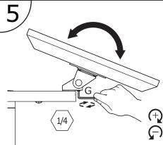
Adjust vertical tilt resistance on tilter head.
