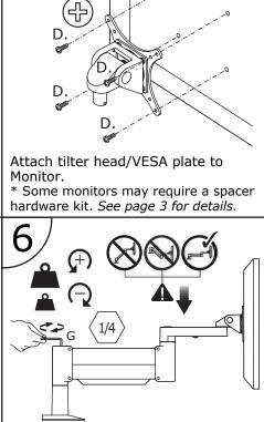
Put arm in horizontal position and rotate wrench CLOCKWISE to WEAKEN arm until monitor stays wherever it is placed. See page 2 for more detailed instructions.
