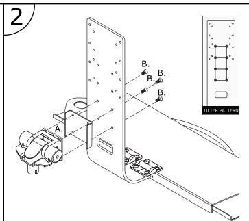
Slide rotation prevention bracket (A) onto face of tilter. Attach backbar to tilter with screws (B) through the tilter hole pattern of your choice.
