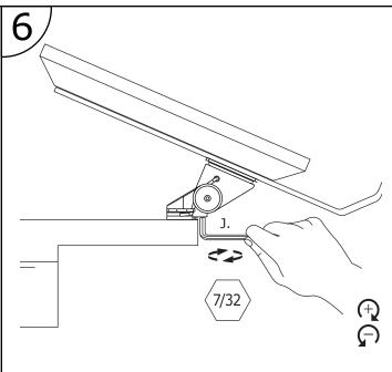
Adjust vertical tilt resistance on tilter head.
