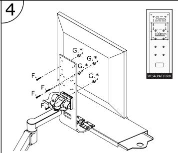
Attach monitor to backbar using screw (F).
