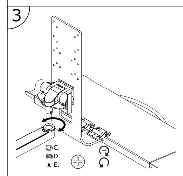
Slide tilter pin into end of arm, secure using dog washer with spacer (C, D, & E).
