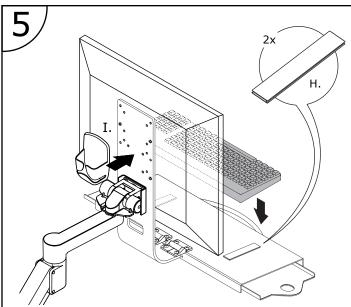
Install mouse holder (I) to backbar in desired location with attached small Velcro strip. Attach large Velcro strips to bottom of keyboard, then attach keyboard to tray in desired location.
