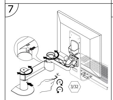
Increase resistance to rotation at articulation points by tightening small set screws. DO NOT OVERTIGHTEN.
