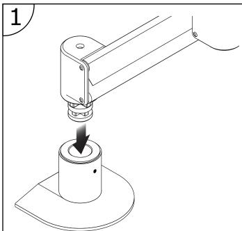
Insert arm pin into completely attached and assembled mount.
