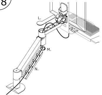
Route monitor cable through arm and install cable caps as shown.
