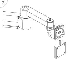
Slide TLT1 rotation stop over the face of the tilter as shown, aligning the holes .
