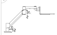
Increase resistance to rotation at articulation points by tightening small set screws.
