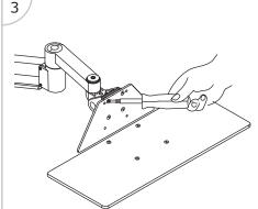
Attach keyboard bracket to tilter using four screws.
