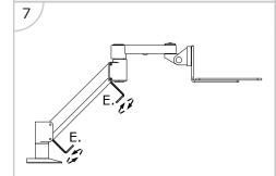
Increase resistance to vertical travel slightly with two hidden set screws on both ends of lifting arm. This control has modest effect and is set only after the gas cylinder has been adjusted to float the keyboard tray.
