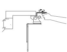
Adjust vertical tilt resistance on tilter head.
