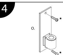
\* Hardware NOT included. The installer must determine exactly what fastener is appropriate for your particular application. If uncertain about mounting procedures contact Ergomart for technical assistance.
