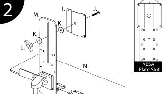
Using the carriage bolt and the plastic knob, fasten the VESA plate to backbar. Position a 1.25" plastic washer on each side of the backbar.
