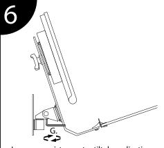
Increase resistance to tilt by adjusting set screw at the point of articulation using wrench (G.)
