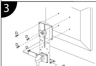
Attach slider VESA plate to LCD with screws (D.)
