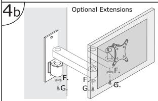
Install optional extensions by sliding extension pins into the wall mount or other extension and secure with dog washer. Slide tilter pin into extension and secure with dog washer.
