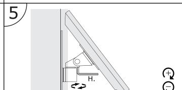
Increase resistance to tilt by adjusting set screw at the point of articulation using wrench.
