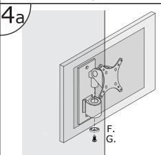
Slide tilter pin into the wall mount and secure with dog washer.  $\,$
